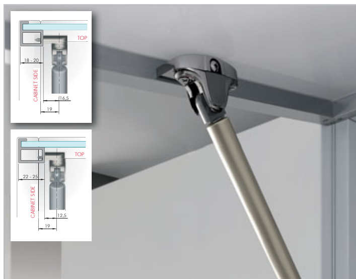
INSTALLATION ON NARROW ALUMINIUM FRAME DOOR
